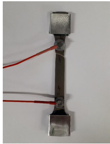
Fig. 2. Tensile specimen with aluminium tabs
